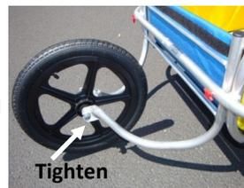
The wheel mount installs between trailer's outer ring and trailer's 2 grooved struts.
