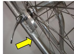
Set the wheel into the dropouts of the frame with the quick release lever to the outside of the trailer. Tighten the nut until the quick release lever can be closed tightly (press lever in, not around in a circle).
